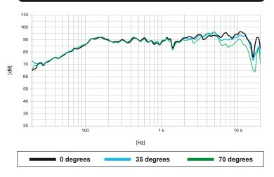
Note: Filtered frequency response measured with loudspeaker standing on infinite baffle in anechoic chamber, 1W @ 1m using filter FD-2CXFe
