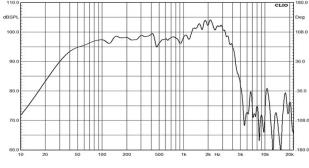
Frequency response measured in a 1200 litre sealed box @ 2,83 v - 1m, 2  $\pi$
