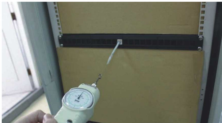
Lock Bar Tension Testing (15kgs)
